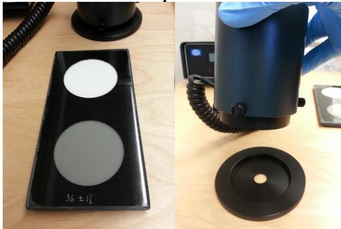
Figure 6.2: Left: Calibration plate (grey and white spaces and). Right: circular mask for holding 25mm filters.
