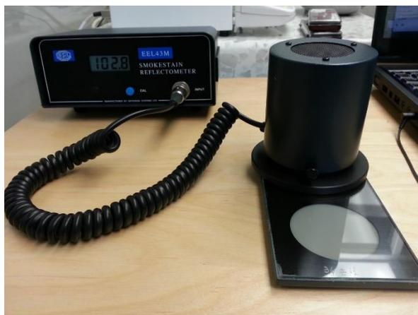
**Figure 6.1: Diffusion Systems SSR (left) and calibration plate with optical unit (right).**
