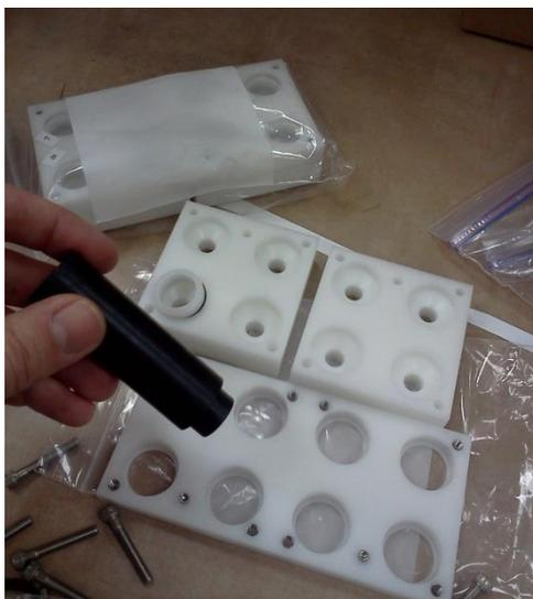
**Figure 3.** Foreground: a disassembled SPARTAN cartridge showing the two top 2x2 blocks as well as the bottom 2x8 block.
