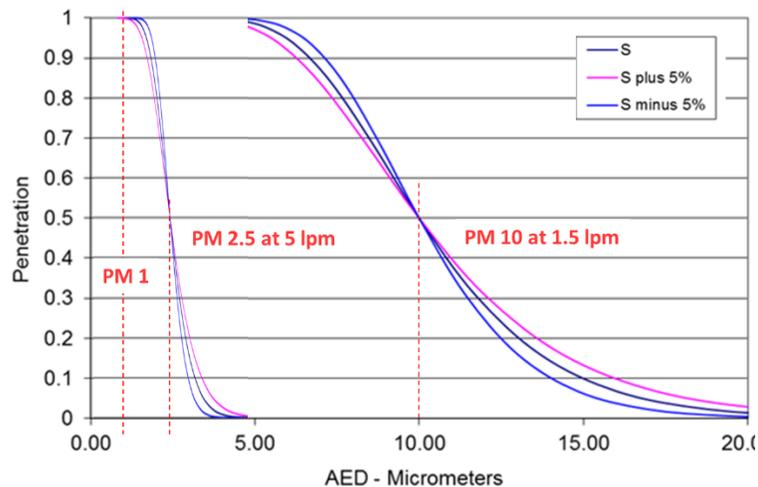
**Figure 5:** Cyclone inlet performance at 1.5 and 5.0 lpm, where penetration refers to the fraction of PM at a given size that is able to pass through the cyclone inlet.
