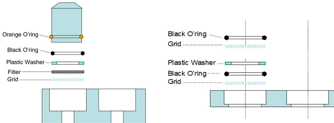
**Figure 1.** Cartridge assembly scheme. Left is TOP half containing the Teflon filters
