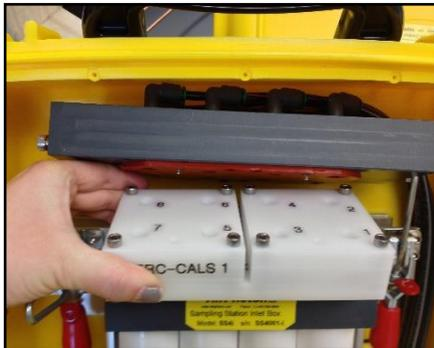
Figure 4: Inserting the cartridge into the sampling station - numbers 1, 3, 5, and 7 should be facing outward
