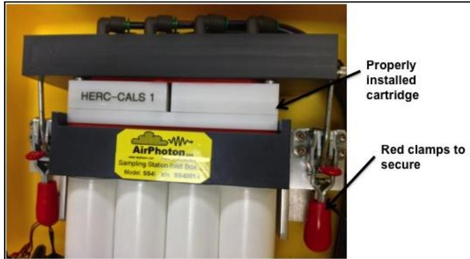
Figure 5: Example of a properly installed cartridge
